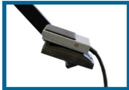
Delay- test starts when delay pedal on the brake pedal is pressed down and stops when pedals are released.
